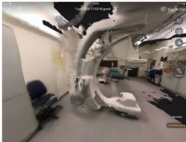
Figure 1. Print screen of the generated 3D mesh of the operating room using Structure sensors and the app Canvas.
