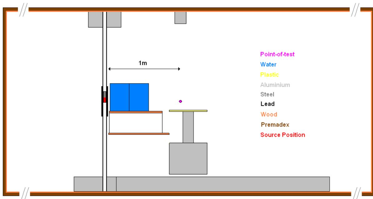
Figure 1: Simulated workplace neutron field at PHE
